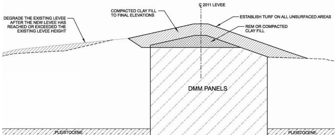
Figure 13. Typical LPV 111 Levee Cross Section (Bertero et al., 2012).
