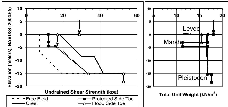
Figure 12. Design undrained shear strength and total unit weight, Reach 12B (Cooling et al., 2012).
