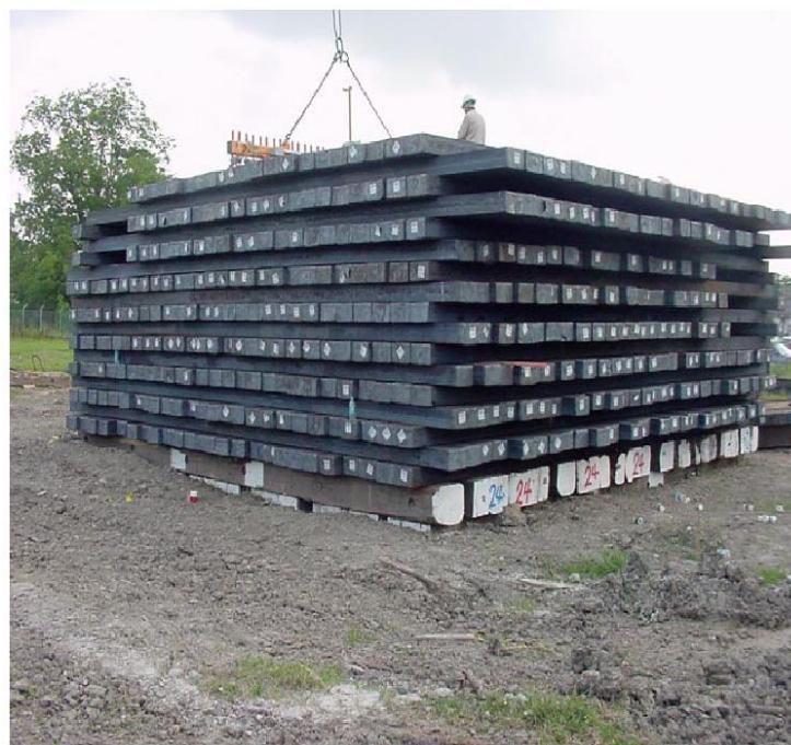
Photograph 2. Cell A fully loaded with 1 million kilograms of steel ( $177 \text{ kN/m}^2$ ).
