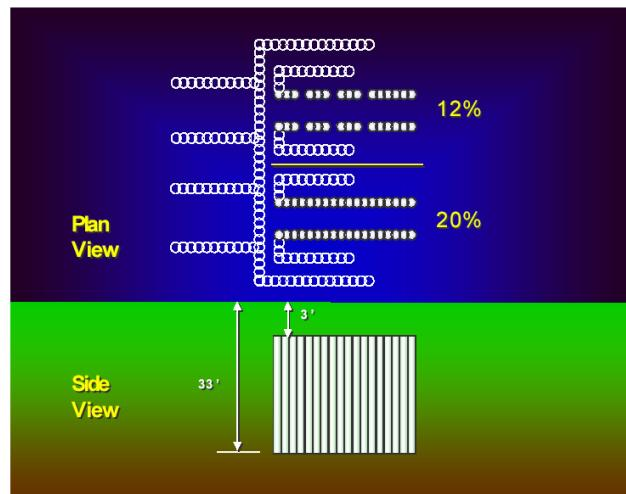
Figure 4. As-built cell configuration with 12% and 20% replacement ratios.
