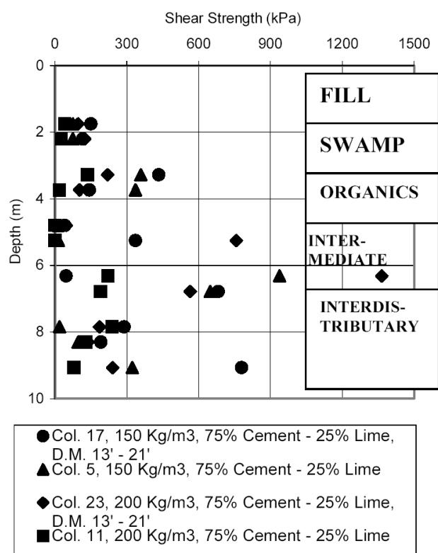
Figure 3. Shear test results on core samples.
