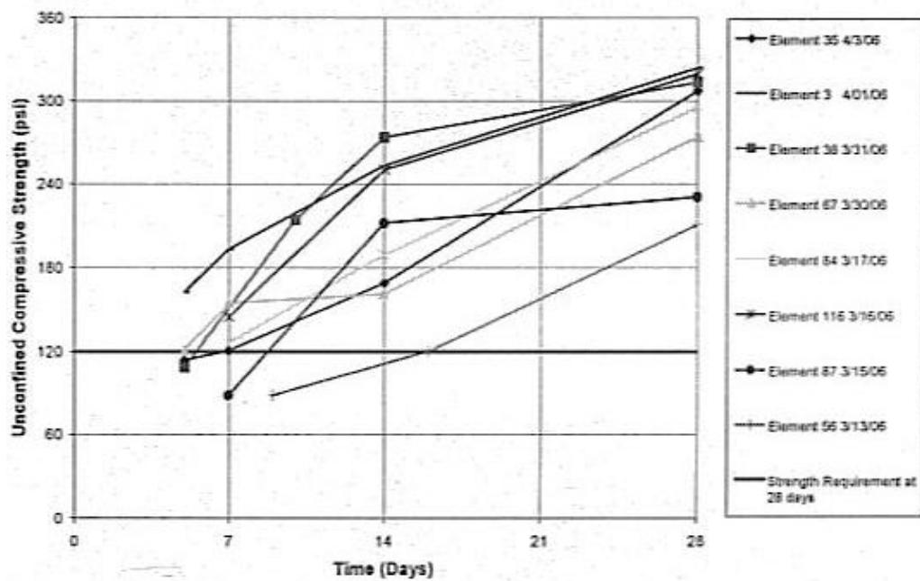
Figure 9. Wet grab sample results, upper 3.3 m, Orleans Avenue Canal, New Orleans ( $1,000 \text{ kPa} \equiv 145 \text{ psi}$ ).
