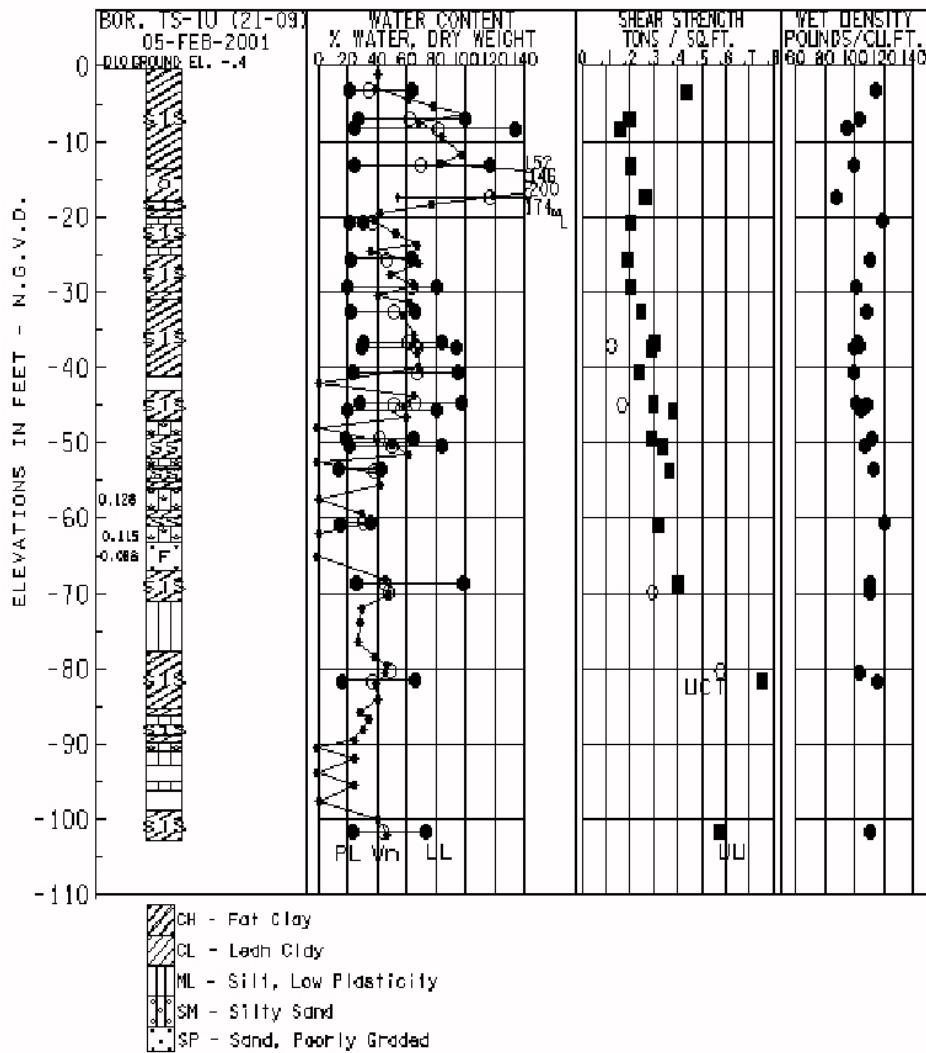
Figure 1. Soil properties obtained from one 127 mm diameter, undisturbed boring (Imperial Units).
