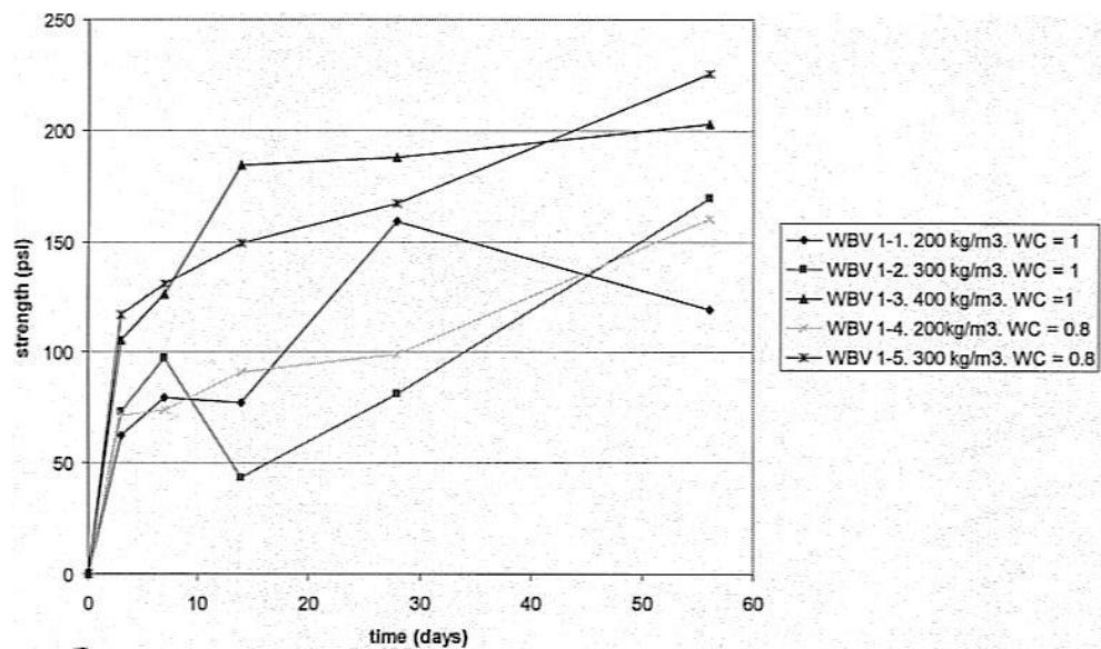
Figure 5. Westwego Pump Station, 56-day bench scale results of the upper 7.5 m (Woodward, 2008) ( $1,000 \text{ kPa} \equiv 145 \text{ psi}$ ).
