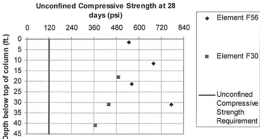
Figure 10. Orleans Avenue, in-situ column coring results at 28 days (Woodward, 2006) ( $1,000 \text{ kPa} \equiv 145 \text{ psi}$ ) ( $1 \text{ m} \equiv 3.28 \text{ ft}$ ).
