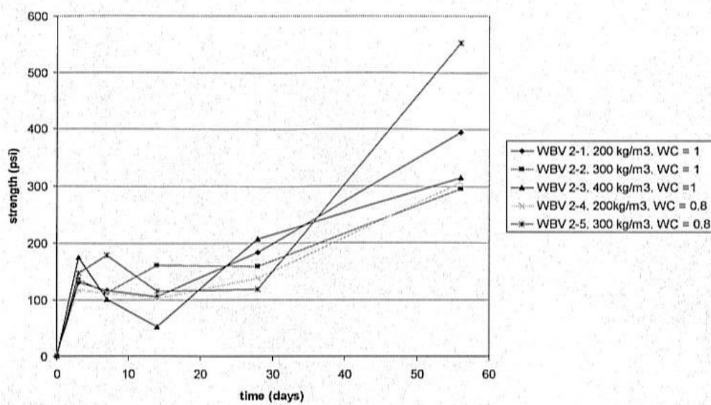
Figure 6. Westwego Pump Station, 56-day bench scale results at 8.4 to 24 m (Woodward, 2008) ( $1,000 \text{ kPa} \equiv 145 \text{ psi}$ ).
