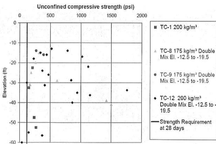
Figure 11. Unconfined compressive strength results of in-situ test columns, 17<sup>th</sup> Avenue Canal, New Orleans ( $1,000 \text{ kPa} \equiv 145 \text{ psi}$ ) ( $1 \text{ m} \equiv 3.28 \text{ ft}$ ).
