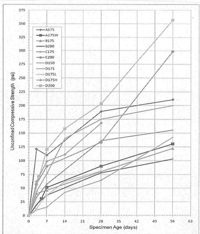
Figure 7. Bench scale test results, Plaquemines Parish Homeplace Levee Setback (Woodward, 2006) ( $1,000 \text{ kPa} \equiv 145 \text{ psi}$ ).
